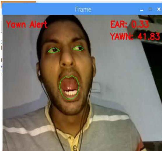
**Fig 7: Yawn detection with alert**
