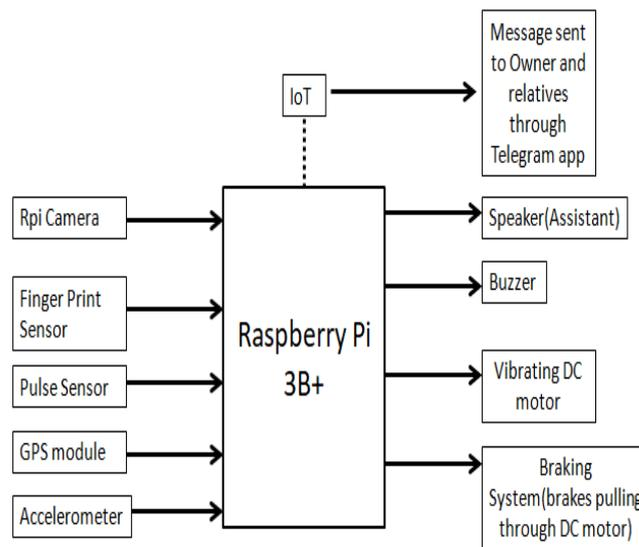
Fig2: Block Diagram of the Project
