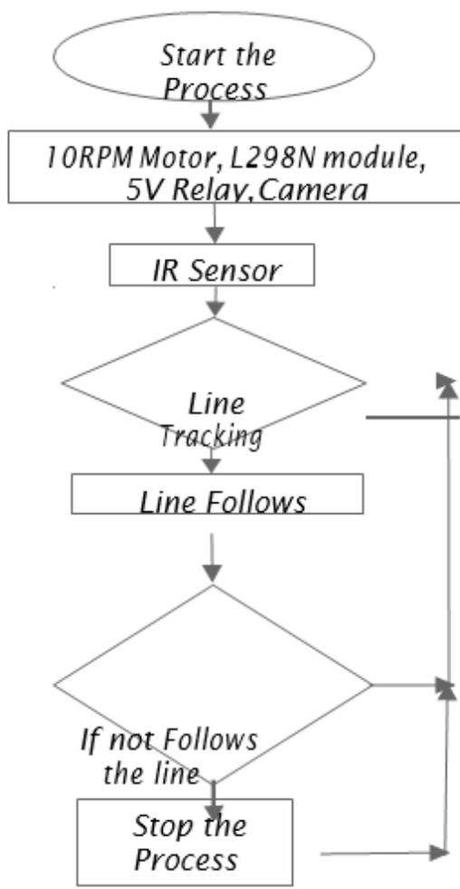
Figure 7: System Operation
