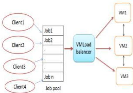
Fig. 4 ESCE (Equally Spread Current Execution) Load Balancing Algorithm (Durgesh& Anand,2015)
