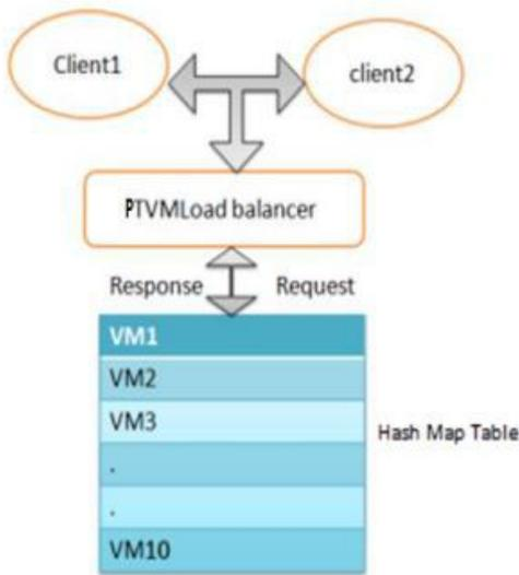
Fig. 3 Throttled Load Balancing Algorithm (Durgesh&Anand , 2015)
