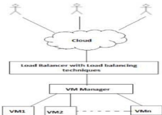
Fig.1 General Structure of Load balancing in Cloud Environment (Garima& Rama, 2015)
