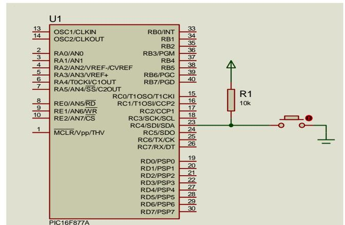
Figure 7: Push Button Sinking current
