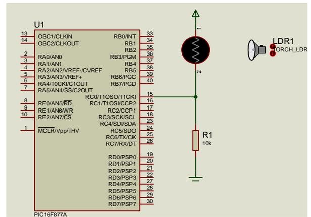
Figure 5: Is one of the lights dependent resistor (LDR) interface and how is calculated
