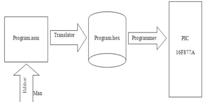
Figure 2: Microcontroller programming process
