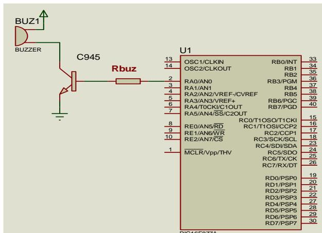
Figure 6: Transistor driven Buzzer
