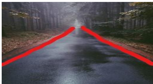
Figure 6 shows Lane Detection in rainy, foggy road
